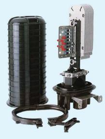
OFC Optical Closure are designed for easy assembly and re-entry in the external plant installation. The water-proof and rugged construction makes these closures perfect for the extreme plant environment. OFC-DB closure are equiped with patch panel and allows branching and interconnection to be done in the closure, eliminating the used of distribution unit.
